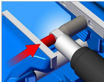
**Assembled tool together with the shock is put into the vice. Bushing is now pressed out of the shock with use of the vice. Bushing is pushed into the bigger part of tool, from where it can be easily removed.**
