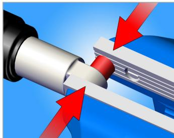
**New bushing is set parallelly next to the opening on the shock and put together in the vice. With use of the vice, bushing is pressed into the shock.** • Novo puščalo paralelno postavimo na odprtino na ohiju amortizerja in skupaj vstavimo v primež. Z enakomernim stiskanjem poskrbimo da je puščalo v celoti stisnjena v ohiju.
