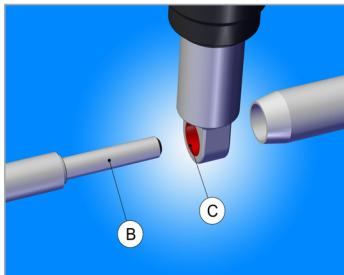
**Size of the pin (B) is chosen upon the bushing (C) size, either 12 mm or 12.7 mm diameter. Tool is assembled as shown on the picture above .**
